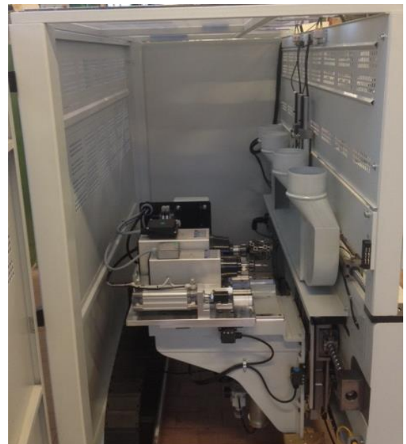
Surround dust collection plus top cover, fully enclosed energy chain
