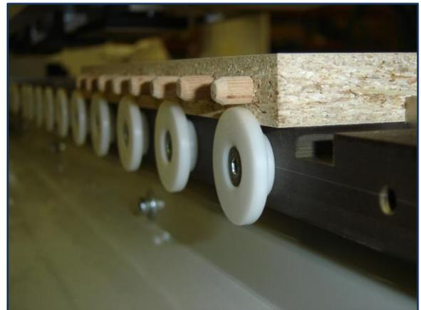
Reference fence is standard with offset PVC discs. The advantage of this type of reference system is that it is not affected by dust plus the machine can bore to the edge.
