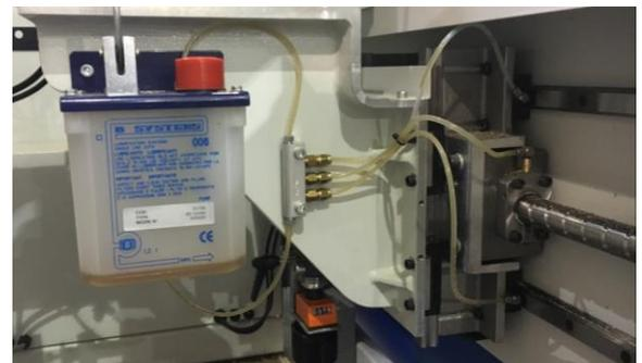
Central lubrication from one pump. Movement of the carriage is on linear rails with square guides and transmission by precision ball screw, which allows precise control. Manual Z axis.
